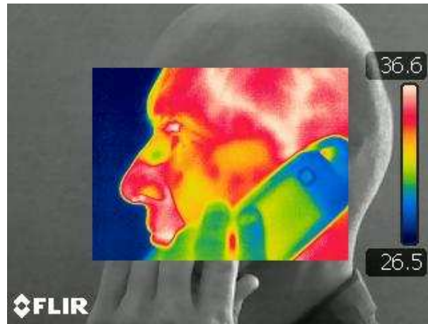
Figure 4: Example how the same photo looks recorded by Thermographic camera
